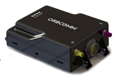
The ST 9100 is a flexible, robust, and programmable dual mode satellite-cellular terminal. It is ideal for remotely monitoring and controlling fixed and portable assets in industries as diverse as transportation, oil and gas, utilities, maritime and more. The versatile, environmentally sealed ST 9100 is ideal for rugged environments in the world's most remote areas.
