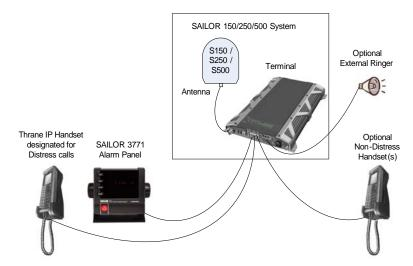
**To make a Distress call**: Push and hold the red button on the alarm panel for 5 seconds. When the Distress IP Handset rings, pick up the phone. You are now put through to the nearest rescue centre. Follow the procedure for Voice Distress calls.
